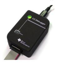
This application note contains hints for using the CC Debugger interface together with a Merifix test fixture, to make a self-contained programming fixture suitable for use in the engineering lab or in low-volume production.
